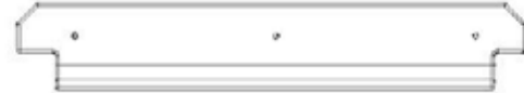
E04 PANNEAU DE REBORD - W4L18696 (x1) 1 7/16 po x 3 3/8 po x 19 15/16 po (36x86x507)
