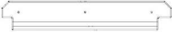
E03 PANNEAU DE REBORD - W4L18695 (x1) 1 7/16 po x 3 3/8 po x 19 15/16 po (36x86x507)
