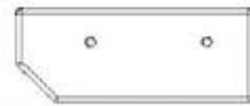
J12 PANNEAU DE REBORD - W4L18816 (x1) 15/16 po x 1 15/16 po x 4 15/16 po (24x50x126)
