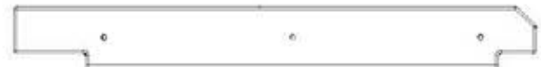
E13 PANNEAU DE REBORD - W4L18719 (x1) 15/16 po x 2 15/16 po x 21 3/4 po (24x74x553)
