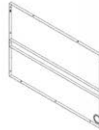
G9 CORNER CABINET BACK PANEL ASSEMBLY R - A4M03043 (x1) 1 3/16"x33 3/8"x47 13/16" (30x848x1215)
