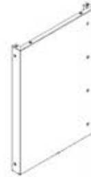
G7 RIGHT CORNER CABINET SIDE WALL ASSEMBLY R - A4M03041 (x1) 2 9/16"x23 3/8"x33 3/8" (65x594x848)
