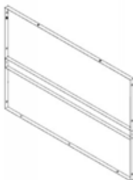
G4 CORNER CABINET BACK PANEL ASSEMBLY L - A4M03033 (x1) 1 3/16"x33 3/8"x47 13/16" (30x848x1215)
