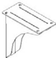
A12 SUPPORT DE PLATEAU DE BAR- A4M03022 (x2) 3 3/4"x7 7/8"x8 7/8" (95x200x225)
