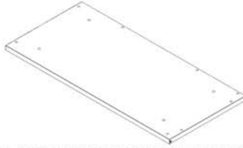
T3 CORNER CABINET MARBLE PANEL ASSEMBLY R - A4M03044 (x1) 1 1/4"x24 1/8"x51 7/8" (32x612x1317)
