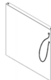
G5 GRILL CABINET SIDE WALL ASSEMBLY M - A4M03059 (x1) 1 3/4"x22 13/16"x23 1/4" (44x579x591)
