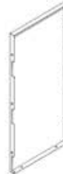
O9 PIZZA OVEN CABINET LEFT BACK PANEL - A4M03065 (x1) 1 3/16"x15 3/16"x33 3/8" (30x386x848)
