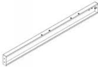
O10 PIZZA OVEN SLIDE UPRIGHT ASSEMBLY - A4M03079 (x1) 1 3/16"x2 15/16"x33 1/4" (30x75x844)
