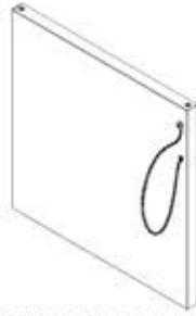
G5 GRILL CABINET SIDE WALL ASSEMBLY M - A4M03050 (x1) 1 3/4"x22 13/16"x23 1/4" (44x579x591)
