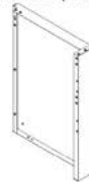
O1 PIZZA OVEN CABINET SIDE PANEL ASSEMBLY R - A4M03064 (x1) 4 3/4"x23 3/8"x33 3/8" (121x594x848)
