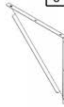
A11 TRIANGLE PANEL - A4M03086 (x2) 13/16"x13 3/4"x13 3/4" (20x350x350)
