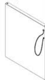
O3 PIZZA OVEN CABINET SIDE PANEL ASSEMBLY M - A4M03077 (x1) 1 3/4"x23 5/16"x26 7/16" (44x592x672)
