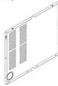
O7 PIZZA OVEN CABINET BACK PANEL ASSEMBLY M - A4M03075 (x1) 1 3/16"x26 7/16"x31 7/16" (30x672x798)
