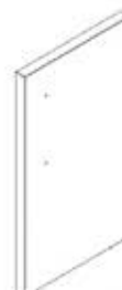
D6 PIZZA OVEN CABINET DOOR ASSEMBLY R - A4M03088 (x1) 1 5/16"x15 9/16"x28 1/8" (34x396x715)
