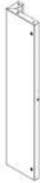
G8 RIGHT CORNER CABINET SIDE WALL ASSEMBLY M - A4M03042 (x1) 3 1/8"x7 1/16"x33 3/8" (80x180x848)
