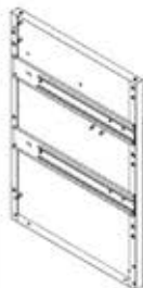
O4 PIZZA OVEN CABINET SIDE PANEL ASSEMBLY ML - A4M03066 (x1) 2 5/8"x23 3/8"x33 3/8" (67x594x848)
