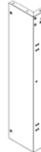
G3 LEFT CORNER CABINET SIDE WALL ASSEMBLY M - A4M03031 (x1) 3 1/8"x7 1/16"x33 3/8" (80x180x848)
