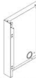
S1 SINK CABINET SIDE PANEL ASSEMBLY L - A4M03094 (x1) 4 3/4"x23 3/8"x33 3/8" (121x594x848)
