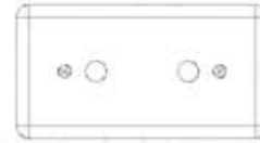
V01 LATCH BLOCK - W4L19241 (x1) 1 1/4"x1 1/4"x2 3/8" (32x32x60)
