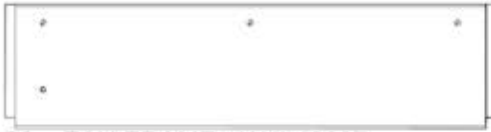
D02 FAN FRAME - W4L19237 (x1) 1 7/16"x5 1/4"x20 13/16" (36x134x529)
