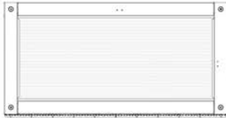
WA01 WINDOW ASSEMBLY - W2A04074 (x1) 1 7/8"x19 5/8"x39 3/16" (48x498x996)
