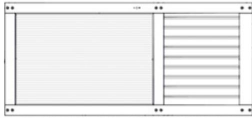
DA01 DOOR ASSEMBLY - W2A04072 (x1) 1 7/8"x36 9/16"x80" (48x928x2032)
