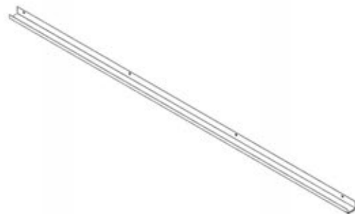
G04 GUTTER - A4M01999 (x2) 1 9/16"x1 15/16"x79 3/8" (40x50x2017)
