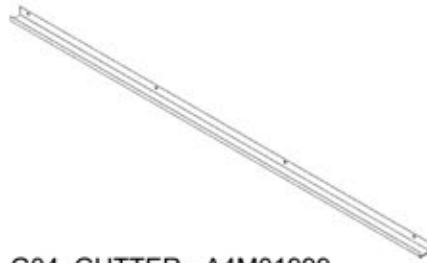
G04 GUTTER - A4M01999 (x1) 1 9/16"x1 15/16"x79 7/16" (40x50x2017)
