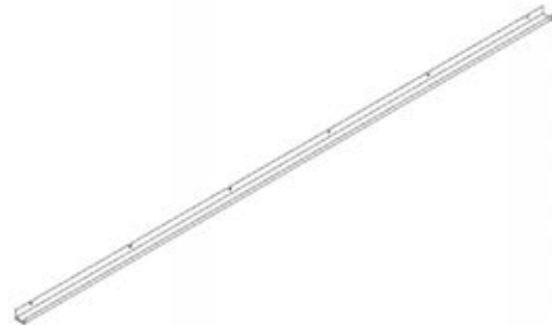
G01 GUTTER - A4M01993 (x2) 1 9/16"x1 15/16"x108 13/16" (40x50x2764)
