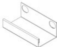
G05 GUTTER SPLICE - A4M02004 (x2) 1 7/16"x2 1/16"x3 15/16" (36x52.5x100)
