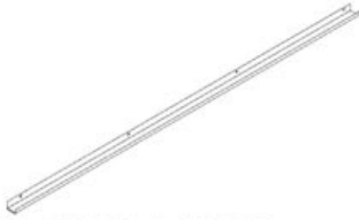
G03 GUTTER - A4M01998 (x1) 1 9/16"x1 15/16"x79 7/16" (40x50x2017)
