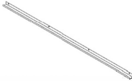
G04 GOUTTIÈRE - A4M01999 (x1) 1 9/16"x1 15/16"x79 7/16" (40x50x2017)
