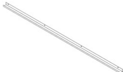
G04 GUTTER - A4M01999 (x2) 1 9/16"x1 15/16"x79 3/8" (40x50x2017)
