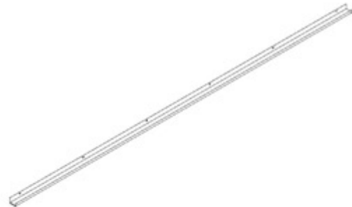
G01 GUTTER - A4M01993 (x2) 1 9/16"x1 15/16"x108 13/16" (40x50x2764)
