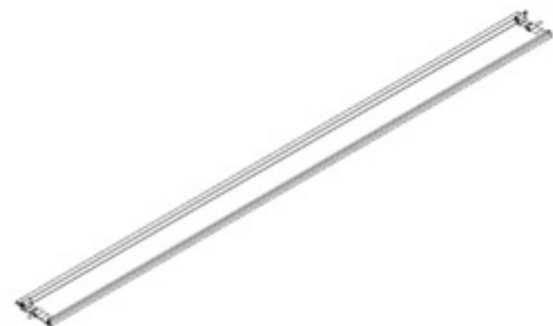
L01 LOUVER ASSEMBLY - A4M01995 (x24) 1 11/16"x7 5/8"x114 5/16" (42x194x2904)
