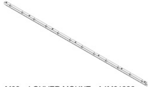
M03 LOUVER MOUNT - A4M01996 (x1) 1"x1 15/16"x79 5/16" (25x49x2015)
