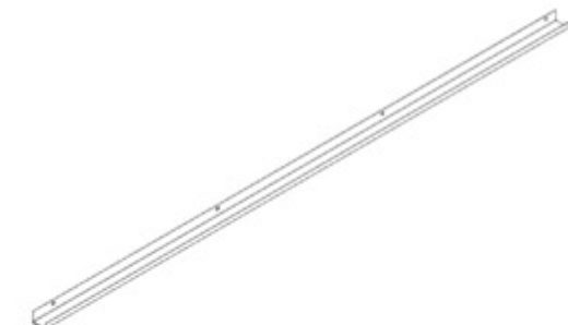
G03 GUTTER - A4M01998 (x2) 1 9/16"x1 15/16"x79 3/8" (40x50x2017)
