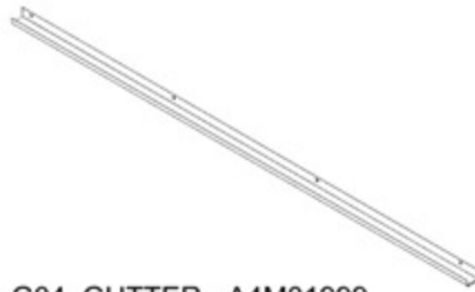
G04 GUTTER - A4M01999 (x1) 1 9/16"x1 15/16"x79 7/16" (40x50x2017)
