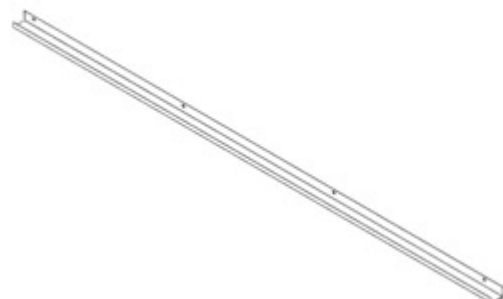
G04 GUTTER - A4M01999 (x2) 1 9/16"x1 15/16"x79 7/16" (40x50x2017)
