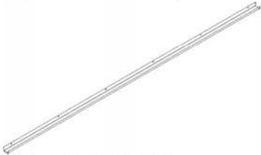
G01 GUTTER - A4M01993 (x2) 1 9/16"x1 15/16"x108 7/8" (40x50x2764)
