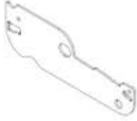
L02 LOUVER DRIVE SIDE PLATE - A4M02134 (x1) 1/16"x2 3/16"x6 9/16" (2x55x167)
