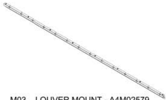
M03 LOUVER MOUNT - A4M02579 (x1) 1"x1 15/16"x92 13/16" (25x49x2357)
