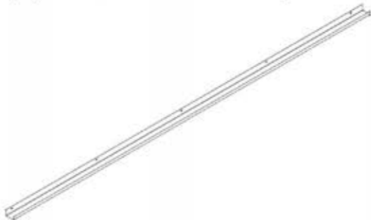
G03 GUTTER - A4M02571 (x2) 1 9/16"x1 15/16"x92 7/8" (40x50x2359)
