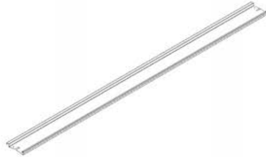
L01 LOUVER ASSEMBLY - A4M01995 (x28) 1 11/16"x7 5/8"x114 5/16" (42x194x2904)
