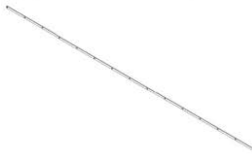
F02 LOUVER TIE STRAP - A4M02573 (x4) 1/8"x5/8"x94 7/8" (3x16x2410)
