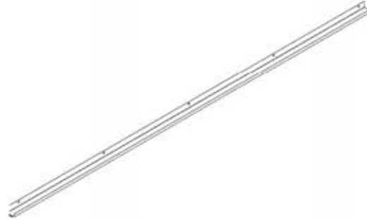
G02 GUTTER - A4M02570 (x2) 1 9/16"x1 15/16"x92 7/8" (40x50x2359)
