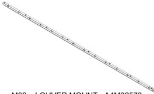
M02 LOUVER MOUNT - A4M02578 (x1) 1"x1 15/16"x92 13/16" (25x49x2357)
