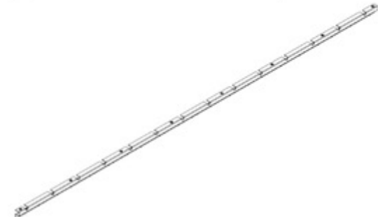
M01 LOUVER MOUNT - A4M02577 (x2) 1"x1 15/16"x92 13/16" (25x49x2357)
