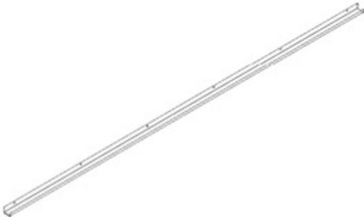
G01 GUTTER - A4M01993 (x2) 1 9/16"x1 15/16"x108 7/8" (40x50x2764)
