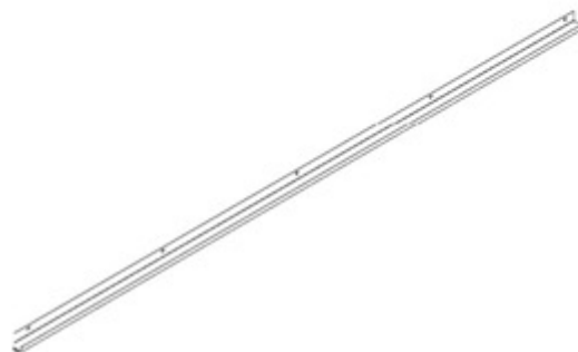
G02 GOUTTIÈRE - A4M02570 (x2) 1 9/16"x1 15/16"x92 7/8" (40x50x2359)
