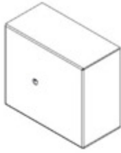
F07 COUVERCLE - A4M02228 (x1) 1 9/16"x2 7/8"x3 1/4" (39.5x73x82)
