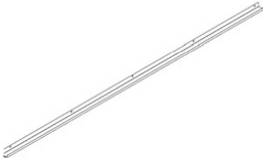
G02 GUTTER - A4M02570 (x2) 1 9/16"x1 15/16"x92 7/8" (40x50x2359)
