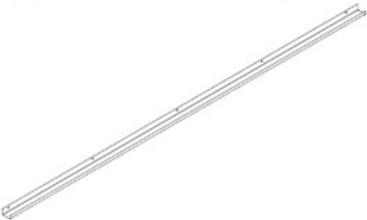
G03 GUTTER - A4M02571 (x2) 1 9/16"x1 15/16"x92 7/8" (40x50x2359)
