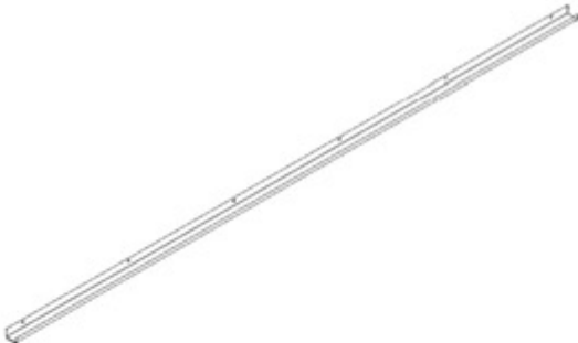
G01 GUTTER - A4M01993 (x2) 1 9/16"x1 15/16"x108 7/8" (40x50x2764)
