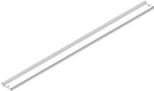
L01 LOUVER - A4M04137 (x28) 1 11/16"x7 3/4"x114 5/16" (42x196.2x2904)
