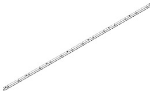
G02 GOUTTIÈRE - A4M02570 (x2) 1 9/16"x1 15/16"x92 7/8" (40x50x2359)
