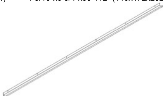
G01 GOUTTIÈRE - A4M01993 (x2) 1 9/16"x1 15/16"x108 7/8" (40x50x2764)
