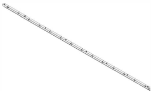
M02 - BATI A PERSIENNES -A4M02578 (x1) 1 "x1 15/16"x92 13/16" (25x49x2357)
