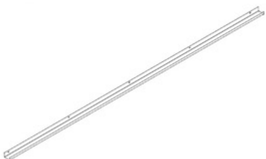
G03 GOUTTIÈRE - A4M02571 (x2) 1 9/16"x1 15/16"x92 7/8" (40x50x2359)
