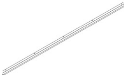
G02 GOUTTIÈRE - A4M02570 (x2) 1 9/16"x1 15/16"x92 7/8" (40x50x2359)
