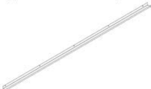
G03 GUTTER - A4M02571 (x2) 1 9/16"x1 15/16"x92 7/8" (40x50x2359)
