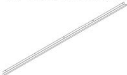
G02 GUTTER - A4M02570 (x2) 1 9/16"x1 15/16"x92 7/8" (40x50x2359)
