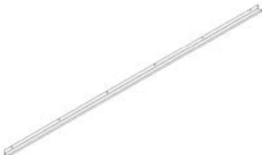
G01 GUTTER - A4M01993 (x2) 1 9/16"x1 15/16"x108 7/8" (40x50x2764)
