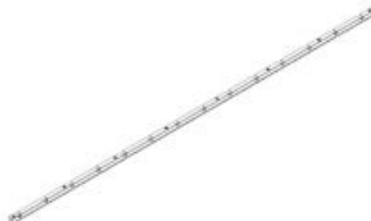
M01 LOUVER MOUNT - A4M02577 (x2) 1"x1 15/16"x92 13/16" (25x49x2357)
