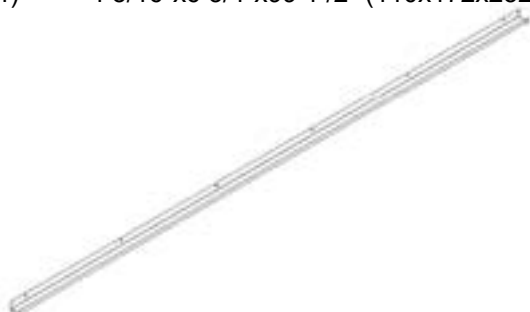
G01 GOUTTIÈRE - A4M01993 (x2) 1 9/16"x1 15/16"x108 7/8" (40x50x2764)
