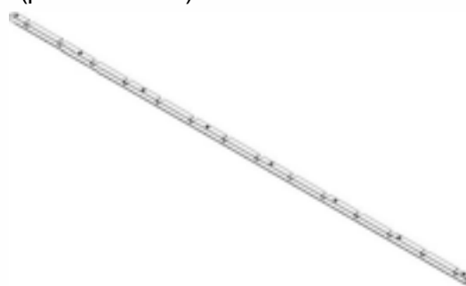
M03-BATI A PERSIENNES-A4M02579 (x1) 1 "x1 15/16"x92 13/16" (25x49x2357)
