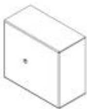
F07 COUVERCLE - A4M02228 (x1) 1 9/16"x2 7/8"x3 1/4" (39.5x73x82)
