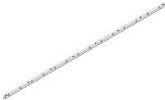
G02 GOUTTIÈRE - A4M02570 (x2) 1 9/16"x1 15/16"x92 7/8" (40x50x2359)
