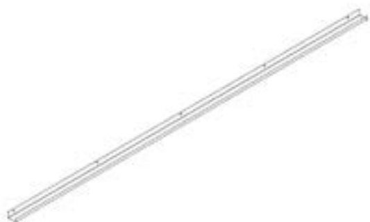
G03 GOUTTIÈRE - A4M02571 (x2) 1 9/16"x1 15/16"x92 7/8" (40x50x2359)
