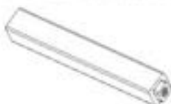
F05 (x1) STOCK CLAVE - A4M02226 1/2"x1/2"x3 3/4" (13x13x95)
