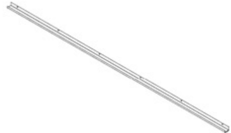
G01 GUTTER - A4M01993 (x2) 1 9/16"x1 15/16"x108 7/8" (40x50x2765)
