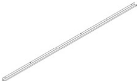
G02 GUTTER - A4M02583 (x4) 1 9/16"x1 15/16"x111" (40x50x2819)
