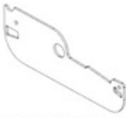
L03 LOUVER SIDE PLATE - A4M04138 (x66) 1/16"x2 3/16"x6 9/16" (2x55x167)
