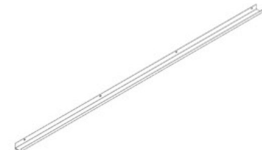
G03 GUTTER - A4M01998 (x2) 1 9/16"x1 15/16"x79 7/16" (40x50x2017)
