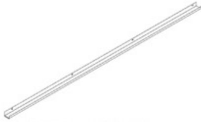
G03 GUTTER - A4M01998 (x1) 1 9/16"x1 15/16"x79 7/16" (40x50x2017)
