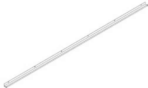
G01 GUTTER - A4M01993 (x2) 1 9/16"x1 15/16"x108 7/8" (40x50x2765)
