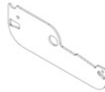
L03 LOUVER SIDE PLATE - A4M04138 (x46) 1/16"x2 3/16"x6 9/16" (2x55x167)
