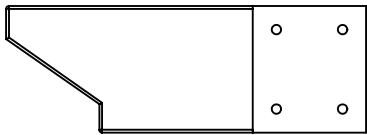
D1 | JOIST END-W4L16247 (1) | 1 7/16"x5 1/4"x15" (36x134x381)
