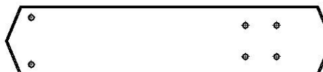
D1 | PLANCHE DE RIVE DU PIGNON - W4L16231 (x4) | 1 7/16 po x 5 1/4 po x 24 3/16 po (36x134x615)
