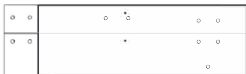
J06 ASSEMBLAGE DE SOLIVE - W2A04078 (x1) 1 7/16 po x 8 7/16 po x 28 7/16 po (36x214x 722)
