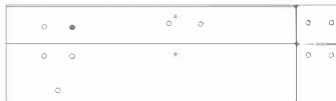
J04 ASSEMBLAGE DE SOLIVE - W2A04080 (x1) 1 7/16 po x 8 7/16 po x 28 7/16 po (36x214x 722)
