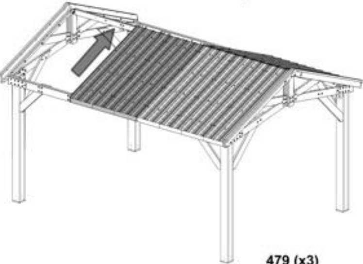
INSTALL ROOF PANEL A, SECTION 2
