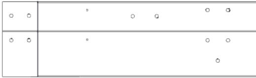
J10 JOIST ASSEMBLY - W2A03820 (x1) 1 7/16"x8 7/16"x28 7/16" (36x214x722)
