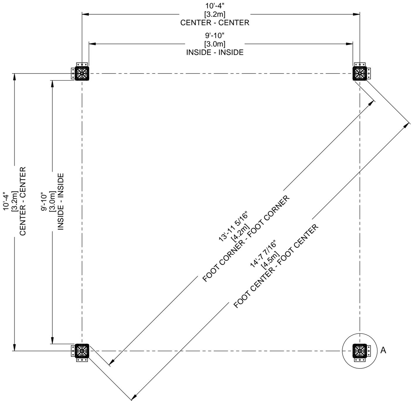
NOTE : LES DIMENSIONS CORRESPONDENT AUX PLAQUES D'ANCRAGE MONTÉES SUR LES POTEAUX, SAUF INDICATION CONTRAIRE.
