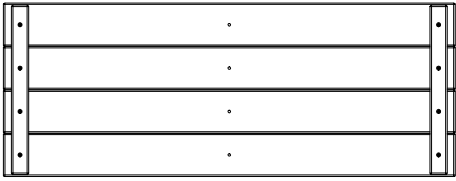
FP1 | BOTTOM FLOOR PANEL - W2A01485 (4) | 1 5/8"x13 1/2"x35 3/8" (40x344x897)
