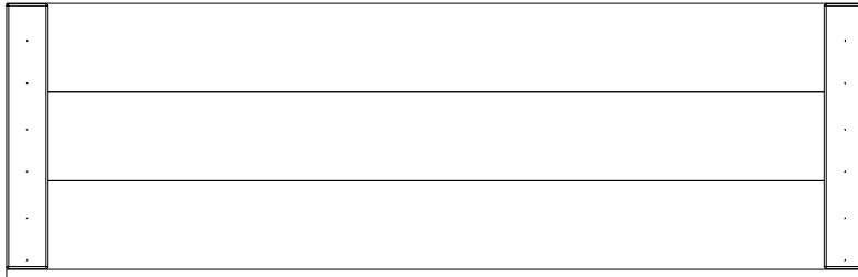
RP2 ROOF PANEL - W2A03794 (x3) 1 5/8"x15 5/8"x59 3/8" (42x396x1241)
