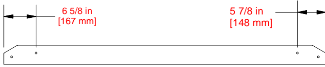
AD02 WALL RAIL - W4L18979 (x2) 1"x3 7/8"x65 3/4" (24x100x1670)
