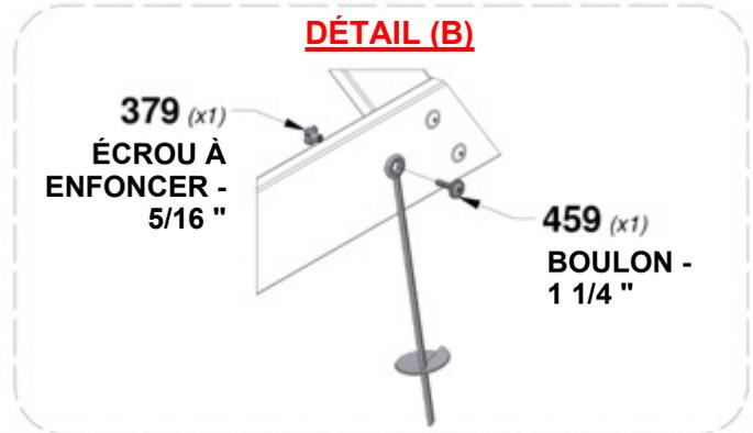
**FAITES PIVOTER LA TARIÈRE EN L'ENFONÇANT DANS LE SOL AUX EMPLACEMENTS INDICUÉS.**
