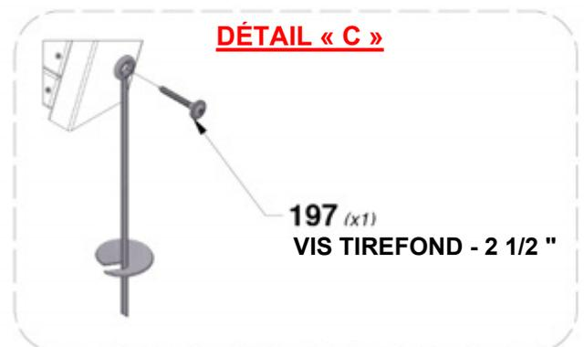
**FAITES PIVOTER LA TARIÈRE EN L'ENFONÇANT DANS LE SOL AUX EMPLACEMENTS INDICUÉS.**
