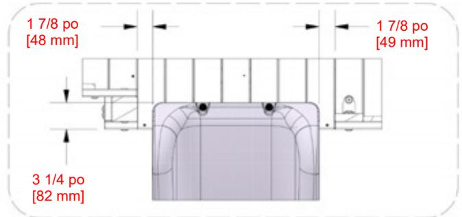
**CENTREZ LE TOBOGGAN DANS L'OUVERTURE EN UTILISANT LES DIMENSIONS INDICUÉES. EN UTILISANT LE TOBOGGAN COMME GABARIT, PERCEZ TROIS (2) TROUS DE 3/8 " [10 mm] À TRAVERS LA PLATEFORME POUR LA QUINCAILLERIE.**
