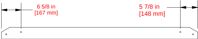
AD02 WALL RAIL - W4L18979 (x2) 1"x3 7/8"x65 3/4" (24x100x1670)
