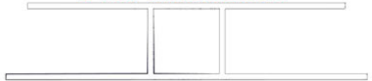
END VIEW OF POLY SPLICE
