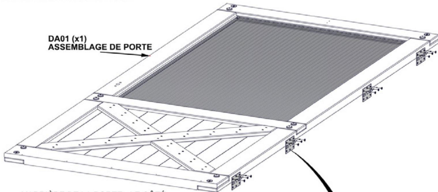
L'ARRIÈRE DE LA PORTE - LE CÔTÉ AVEC LE SUPPORT X
