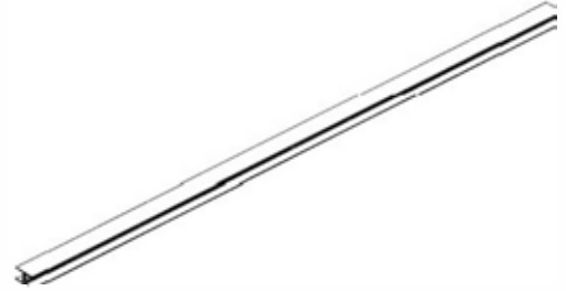
A2 VERTICAL SUPPORT - A4M02039 (x1) 1 15/16"x1 3/16"x57 7/8" (30x50x1470)
