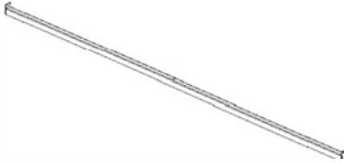
A1 HORIZONTAL BRACE ASSEMBLY - A4M01806 (x2) 1 7/16"x2 5/16"x88" (36x58x2235)
