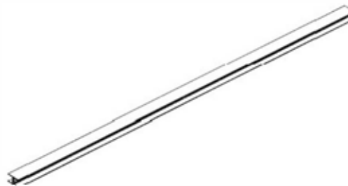
A2 SUPPORT VERTICAL - A4M02039 (x1) 1 15/16"x1 3/16"x57 7/8" (30x50x1470)
