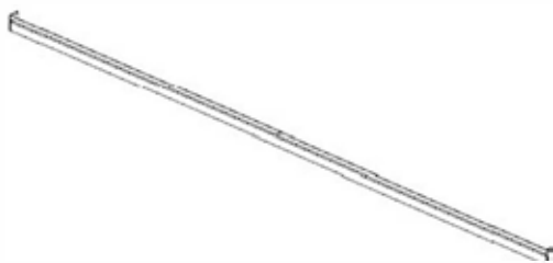
A1 ENSEMBLE DE CONTREVENTEMENT HORIZONTAL - A4M01806 (x2) 1 7/16"x2 5/16"x88" (36x58x2235)
