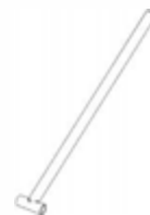
R04 PIVOT ROD - A4M02784 (x1) 1/2"x1 7/16"x12 1/4" (12x36x312)
