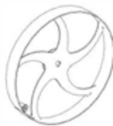
W01 WHEEL ASSEMBLY - A4M02146 (x1) 2 3/8"x7" (x59.7x178)
