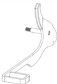
H02 SPROCKET HANDLE ASSEMBLY - A4M02760 (x1) 3 5/8"x4 1/2"x9 5/16" (92x115x236)
