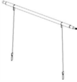
S01 SPINDLE ASSEMBLY - A4M02150 (x1) 1 3/16"x37 5/8" (30x955)
