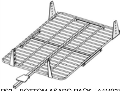
R02 BOTTOM ASADO RACK - A4M02786 (x1) 4 1/4"x18 1/2"x34" (108x470x864)
