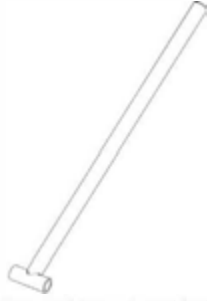
R04 PIVOT ROD - A4M02784 (x1) 1/2"x1 7/16"x12 1/4" (12.0x36x312)
