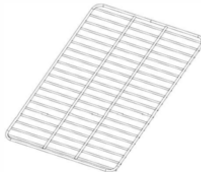
R01 TOP ASADO RACK - A4M02785 (x1) 5/16"x18 3/8"x30 5/16" (8x466x770)
