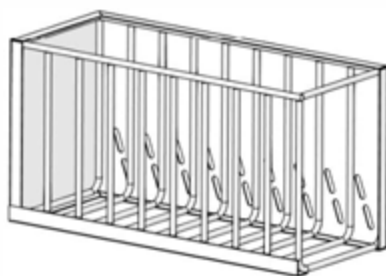
F01 FIRE BOX - A4M02772 (x1) 11 11/16"x9 1/8"x22 1/2" (298x232x572)
