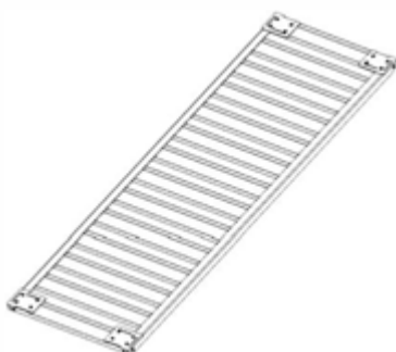
B02 BOTTOM RACK ASSEMBLY - A4M02767 (x1) 1 5/8"x24 1/16"x74 3/4" (40.5x611.5x1898)
