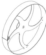
W01 ROUE - A4M02146 (x1) 2 3/8"x7" (59.7x178)
