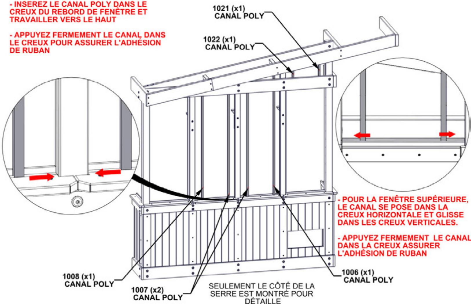
**- POUR LA FENÊTRE SUPÉRIEURE, LE CANAL SE POSE DANS LA CREUX HORIZONTALE ET GLISSE DANS LES CREUX VERTICALES.**
