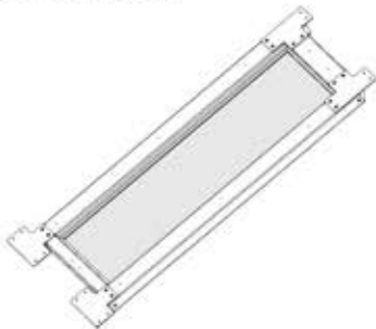
WINDOW ASSEMBLY WITH CLEATS FROM STEP 120
