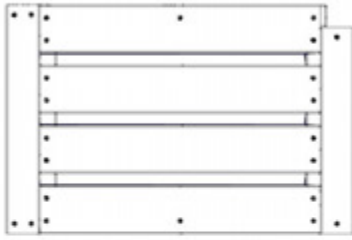
TB07 TABLE ASSEMBLY - W2A04210 (x1) 2 1/16"x16 1/16"x24 7/16" (52x408x620)
