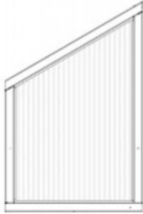
WA04 WINDOW ASSEMBLY - W2A04377 (x1) 1 7/16"x22 3/16"x33 15/16" (36x563x788)
