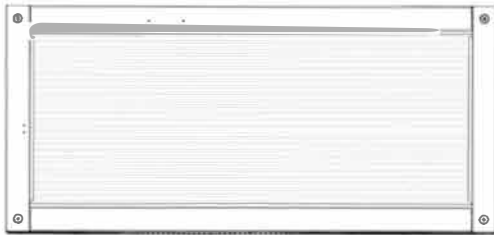
WA07 WINDOW ASSEMBLY - W2A04206 (x2) 1 7/8"x21 13/16"x47 3/16" (48x554x1198)
