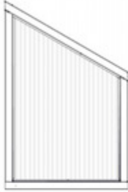
WA03 WINDOW ASSEMBLY - W2A04375 (x1) 1 7/16"x22 3/16"x33 15/16" (36x563x788)
