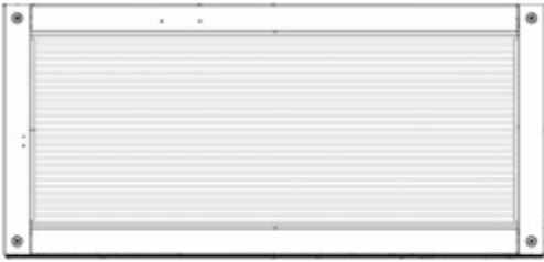
WA07 WINDOW ASSEMBLY - W2A04206 (x1) 1 7/8"x21 13/16"x47 3/16" (48x554x1094)
