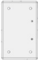
K04 LATCH BLOCK - W4L19789 (x2) 5/8"x3"x4 3/4" (16x76x120)
