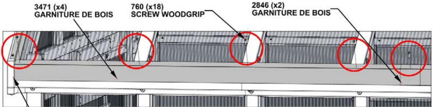
**CENTER SCREWS ON SPLICE COVERS AND ATTACH SCREWS THROUGH TRIM AND SPLICE COVERS.**
