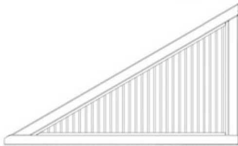
WA01 WINDOW ASSEMBLY - W2A04157 (x2) 1 7/16"x19 11/16"x32 11/16" (36x501x830)
