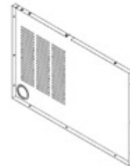
G1 PIZZA OVEN CABINET BACK PANEL ASSEMBLY - A4M03542 (x1) 38 3/4"x26 1/2"x1 3/16" (30x673.5x984)
