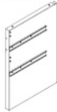
S5 SINK CABINET SIDE PANEL ASSEMBLY M - A4M03567 (x1) 33 3/8"x23 3/8"x2 3/16" (56.2x593x847)
