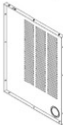
G4 FRIDGE CABINET BACK PANEL ASSEMBLY - A4M03599 (x1) 25 5/16"x33 3/8"x1 3/16" (30x847.2x864)
