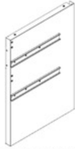
S5 SINK CABINET SIDE PANEL ASSEMBLY M - A4M03567 (x1) 33 3/8"x23 3/8"x2 3/16" (56.2x593x847)
