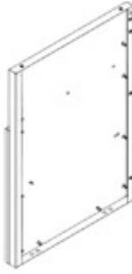
S7 FRIDGE CABINET SIDE PANEL ASSEMBLY L - A4M03597 (x1) 33 7/16"x23 3/8"x2 1/16" (53x594x849.7)
