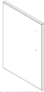
D1 PIZZA OVEN CABINET DOOR ASSEMBLY L - A4M03546 (x1) 28 7/16"x19 5/8"x15/16" (24x498x722.5)
