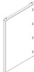
S8 FRIDGE CABINET SIDE PANEL ASSEMBLY R - A4M03598 (x1) 33 3/8"x23 3/8"x1 15/16" (50x594x848.20)
