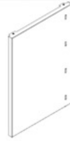
S8 FRIDGE CABINET SIDE PANEL ASSEMBLY R - A4M03598 (x1) 33 3/8"x23 3/8"x1 15/16" (50x594x848.20)
