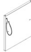
S2 PIZZA OVEN CABINET SIDE PANEL ASSEMBLY M - A4M03545 (x1) 26 1/2"x23 3/8"x1 3/8" (35x593x673.5)
