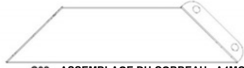
C02 ASSEMBLAGE DU CORBEAU - A4MQ3526 (x1) 21 13/16"x5 1/4"x2 3/4" (70x134x553.5)
