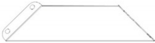
C01 ASSEMBLAGE DU CORBEAU - A4M03525 (x1) 21 13/16"x5 1/4"x2 3/4" (70x134x553.5)
