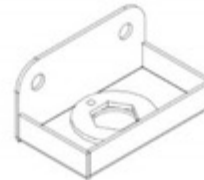
A9 ASSEMBLAGE SUPPORT DE TUYAU - A4M03060 (x2) 1 1/4"x1 7/16"x2 9/16" (31.5x36.5x65)
