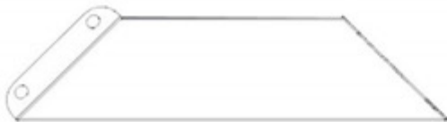
C01 ASSEMBLAGE DU CORBEAU - A4M03525 (x1) 21 13/16"x5 1/4"x2 3/4" (70x134x553.5)
