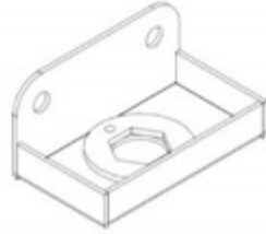
A9 ASSEMBLAGE SUPPORT DE TUYAU - A4M03060 (x1) 1 1/4"x1 7/16"x2 9/16" (31.5x36.5x65)
