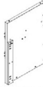
S4 SINK CABINET SIDE PANEL ASSEMBLY R - A4M03563 (x1) 33 3/8"x23 3/8"x2 5/8" (67.00x594.00x848.20)
