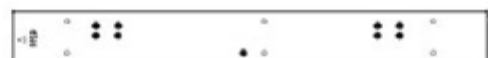
H10 PIZZA OVEN CABINET HINGE CHANNEL ASSEMBLY - A4M03686 (x1) 26 9/16"x2 15/16"x2 1/8" (54.00x74.80x674.00)
