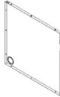
G3 SINK CABINET BACK PANEL ASSEMBLY - A4M03564 (x1) 34 5/16"x33 3/8"x1 3/16" (30.00x847.20x872.00)
