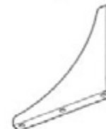
A7 TRIANGLE BRACKET - A4M03708 (x2) 5 7/8"x5 7/8"x9/16" (15.00x150.00x150.00)
