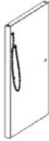
S2 PIZZA OVEN CABINET SIDE PANEL ASSEMBLY M - A4M03545 (x1) 26 1/2"x23 3/8"x1 3/8" (35.00x593.00x673.50)
