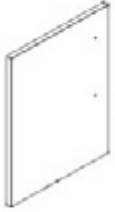
D14 PIZZA OVEN CABINET DOOR ASSEMBLY L - A4M03659 (x1) 28 7/16"x18 7/8"x15/16" (24.00x480.00x722.50)
