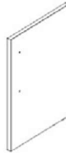
D8 GRILL CABINET DOOR ASSEMBLY R - A4M03590 (x1) 24 13/16"x19 1/16"x15/16" (24.00x484.15x630.00)
