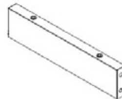
H8 CORNER CABINET HORIZONTAL BEAM ASSEMBLY - A4M03672 (x1) 12 15/16"x3"x1" (25.00x76.50x328.80)
