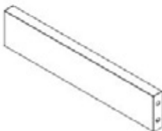
H4 HORIZONTAL BEAM ASSEMBLY L - A4M03575 (x4) 16 1/4"x3 3/8"x1" (25.00x85.00x413.00)
