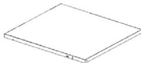
L6 CORNER CABINET SHEFT ASSEMBLY - A4M03680 (x1) 25 5/8"x23 3/16"x1" (25.00x589.00x650.40)
