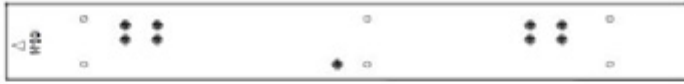
H10 PIZZA OVEN CABINET HINGE CHANNEL ASSEMBLY - A4M03686 (x1) 26 9/16"x2 15/16"x2 1/8" (54.00x74.80x674.00)
