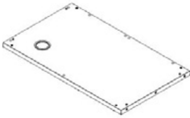
T1 PIZZA OVEN CABINET TABLETOP ASSEMBLY - A4M03543 (x1) 40 3/16"x23 3/8"x1 1/4" (32x594x1020)
