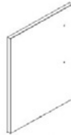
D14 PIZZA OVEN CABINET DOOR ASSEMBLY L - A4M03659 (x1) 28 7/16"x18 7/8"x15/16" (24.00x480.00x722.50)
