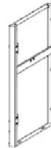
S14 PIZZA OVEN CABINET SIDE PANEL ASSEMBLY - A4M03657 (x1) 26 9/16"x23 3/8"x1 3/8" (35.00x594.00x675.00)
