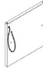
S6 GRILL CABINET SIDE PANEL ASSEMBLY M - A4M03586 (x1) 23 3/8"x22 7/8"x1 3/8" (35.00x581.00x593.00)
