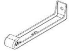
4759 GUTTER HANGER - A4M04759 (x4) 3/4"x1"x4 15/16" (1.9x2.5x12.5)
