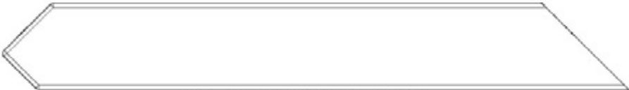
F18 ANGLE BRACE - W4L21307 (x1) 1 7/16"x2 3/8"x17" (36x60x432)
