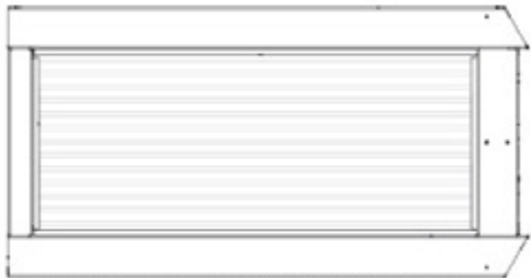
WA05 WINDOW ASSEMBLY - W2A04526 (x1) 1 7/16"x15 1/4"x29 7/16" (36x388x747)
