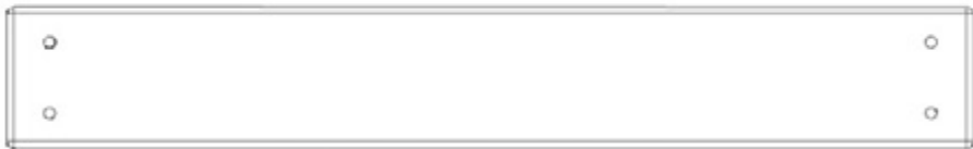
N11 TABLE TOP SPLICE - W4L21304 (x1) 5/8"x2 3/8"x16 1/16" (16x60x408)
