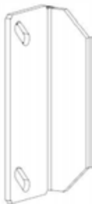
A4M02410 STORM DOOR HANDLE LATCH (x1)
