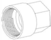
A6P00648 THREADED HOSE FITTING (x1)
