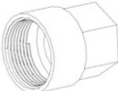
A6P00648 THREADED HOSE FITTING (x1)
