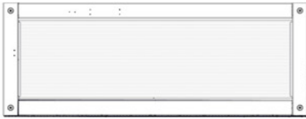
WA01 WINDOW ASSEMBLY - W2A04438 (x1) 1 7/8"x17 1/2"x47 3/16" (48x444x1198)
